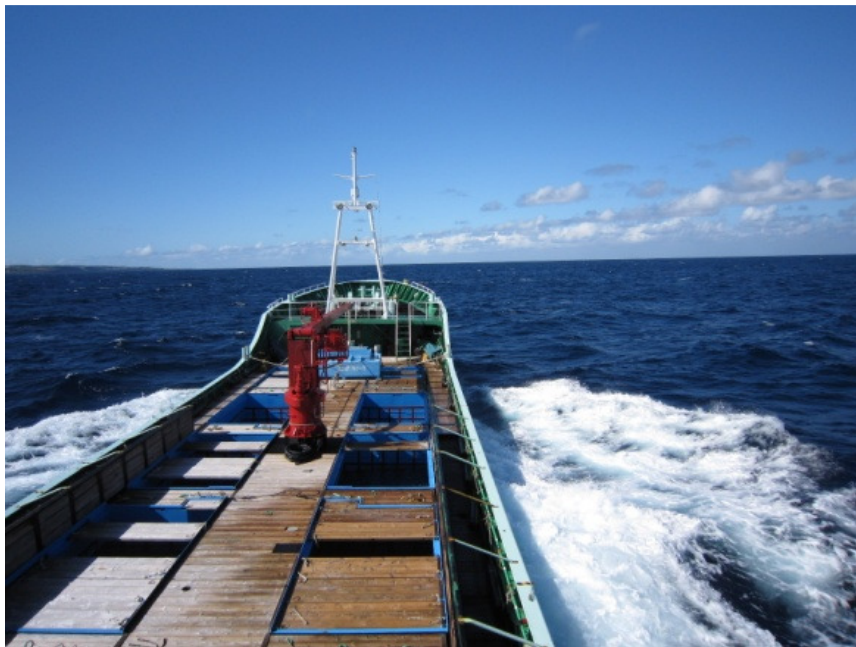
Figure 2. The transport vessel with live fish holding containers for scalloped hammerhead shark ( Sphyrna lewini ) transportation.
