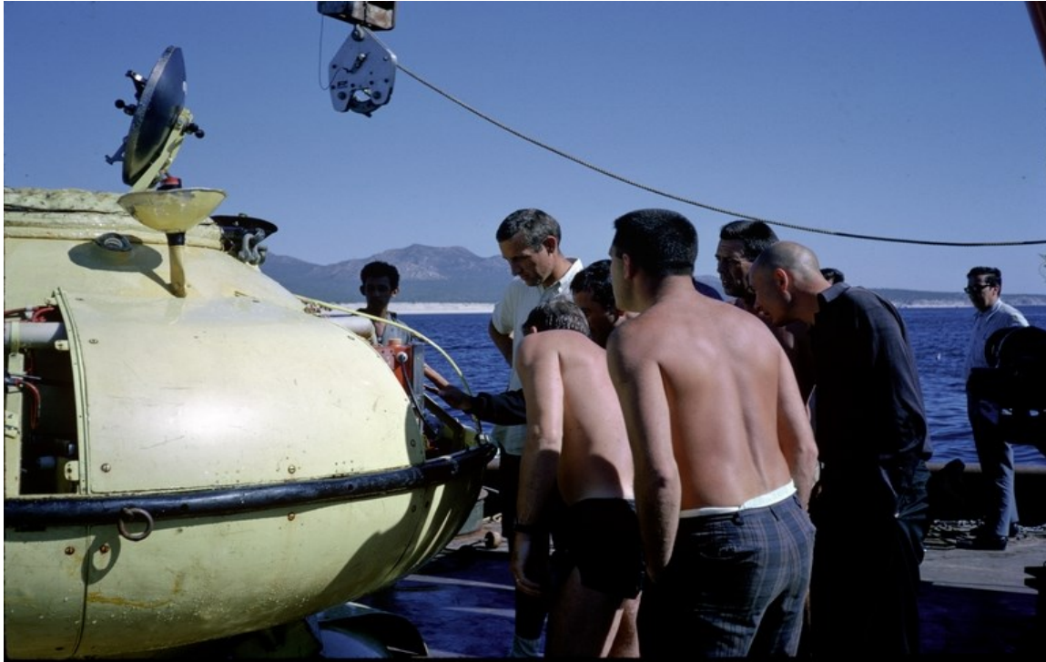
Figure 3. Possibly the same submarine Dr. Richard Rosenblatt dove in 1965. The Jacques Cousteau diving saucer, equipped with a grabber/manipulator, cameras, headlights and underwater jets. The oxygen tank could support two persons for up to 24 hours. Photo: Jimmy Stuart, courtesy of UCSD Digital Library.
