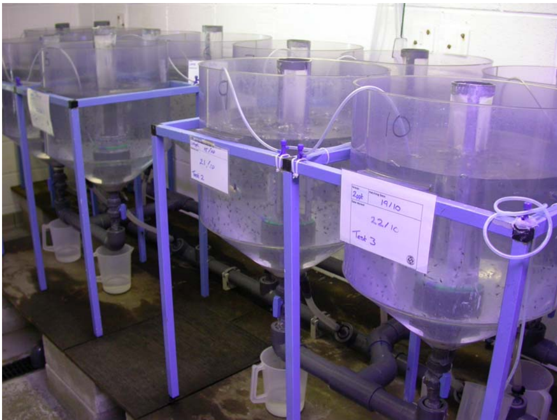
Photo 2. 12 Kreisel cone recirculation system used to rear larvae from hatching through to stage IV.
