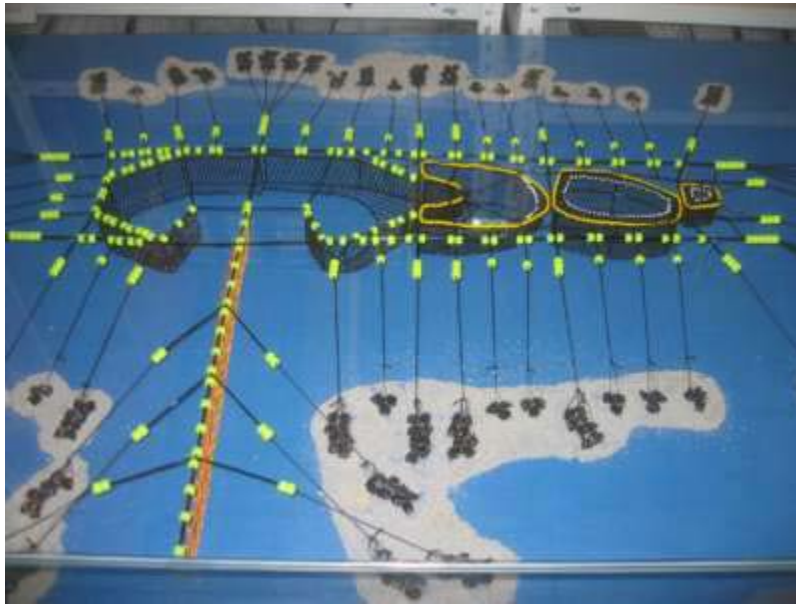
Fig. 2. Typical model of an ‘almadraba’ set-net.
